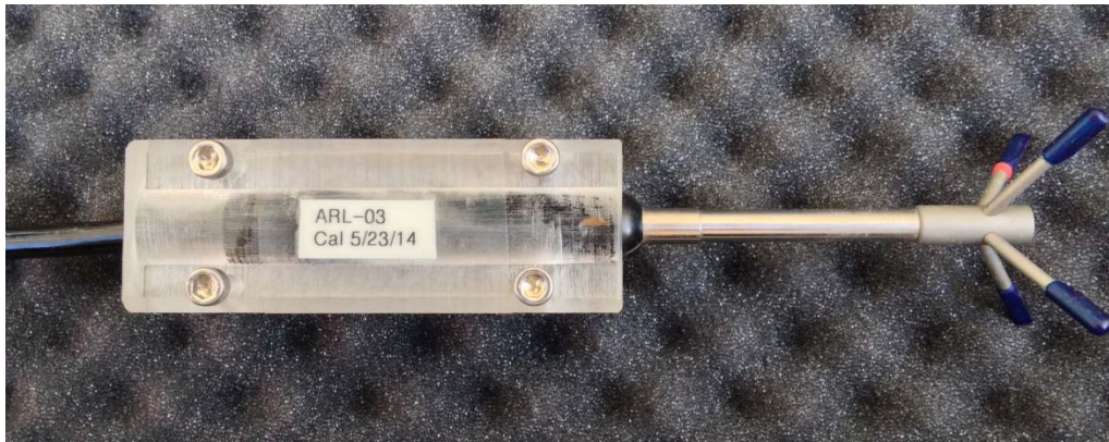
Photo 2-2 ADV in Calibrated Acrylic Block Housing
